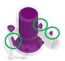
Sectional solidification analysis suggests isolated hot region inside the boss is present even after the revised methoding.
