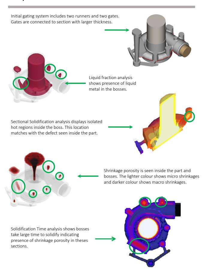
The suggested methoding improvements included a slightly larger central feeder of 90 mm height and 65 mm diameter, with a 10-mm thick insulation sleeve, and a chill on the side boss.
