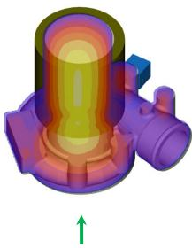
3D solidification simulation and the feed path analysis of the revised methoding show good feeding characteristics, with the feed paths converging inside the feeder.
