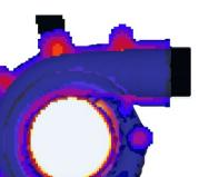
Liquid fraction analysis displays presence of liquid metal inside the part and bosses indicating possibility of shrinkage porosity in these locations.
