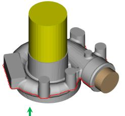
The methoding layout of the part included a central top feeder of height 75 mm and diameter 60 mm, feeding the entire casting.
