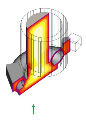
The sectional solidification view shows no isolated hot spot in the boss section which ensures the casting quality.
