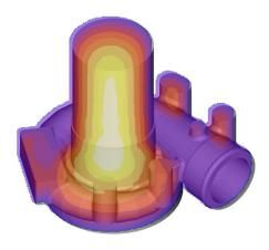
3 D solidification simulation and the sectional view of the current methods design show an isolated shrinkage defect at the external boss section, which matches the defect found in the actual casting.
